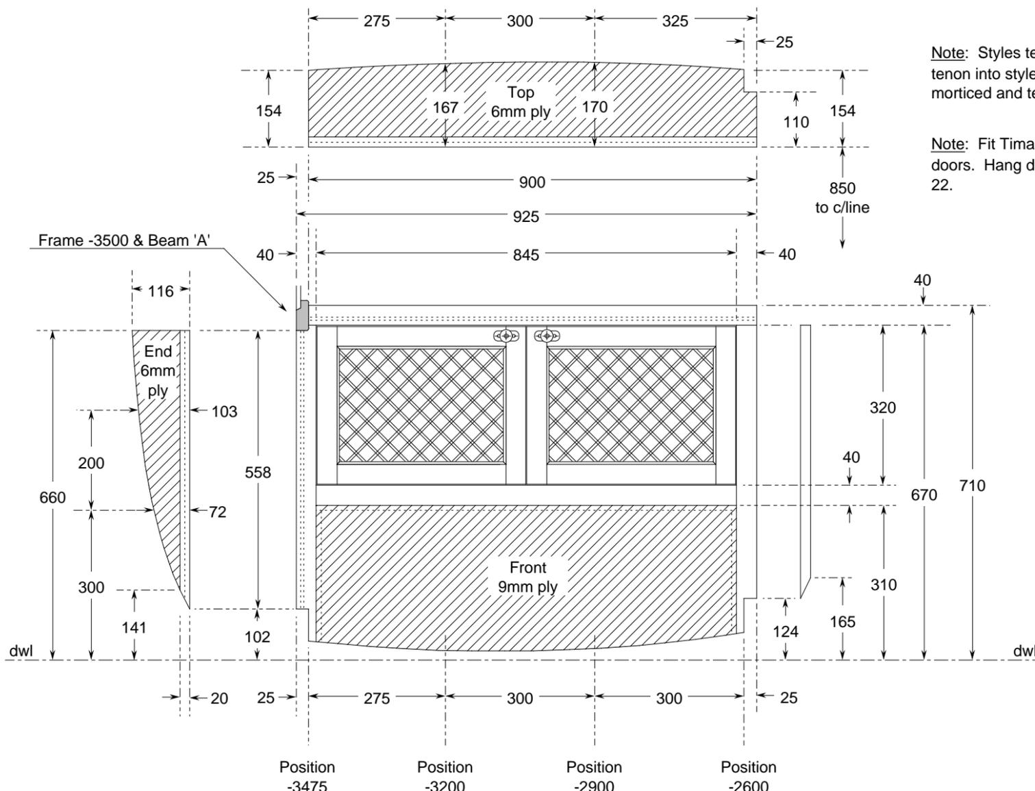
Note: Styles tenon into top rail. Bottom rails tenon into styles. Door rails and styles are morticed and tenoned together.
