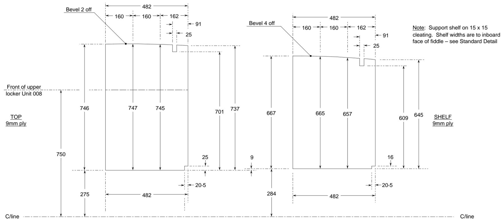
Note: Support shelf on 15 x 15 cleating. Shelf widths are to inboard face of fiddle – see Standard Detail
