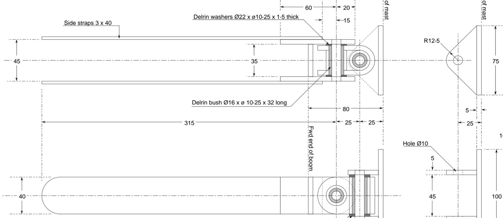
**Note:** Gooseneck material mild steel hot-dip galvanized after fabrication. Gooseneck made from 5mm material (side straps 3mm and bushes as shown). Delrin for bearing bushes and washers. Hole sizes given are after galvanizing - so allow clearance on holes in steel items for galvanizing thickness.
