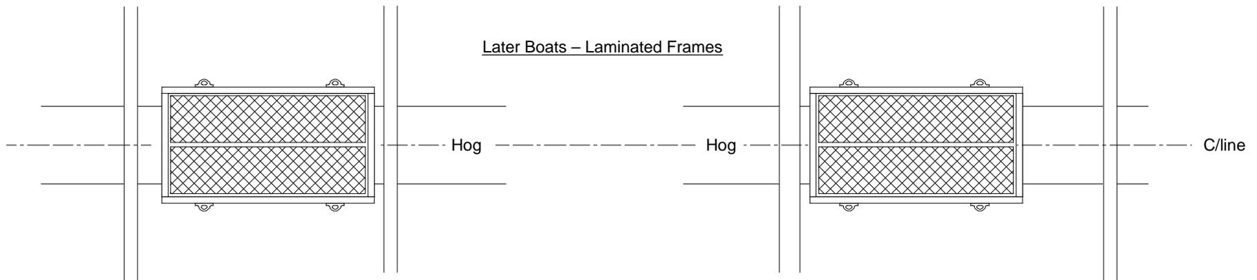
Typical ballast pig = 65 x 90 x 375 = 25kg
