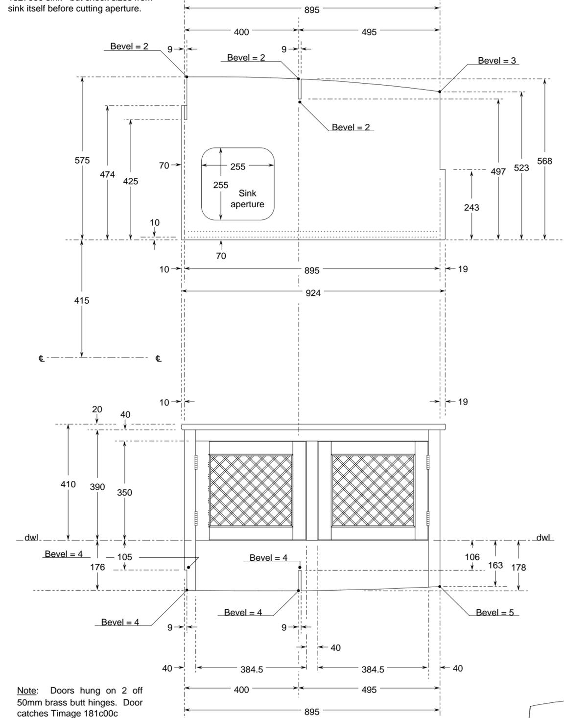
Note: Doors hung on 2 off 50mm brass butt hinges. Door catches Timage 181c00c
