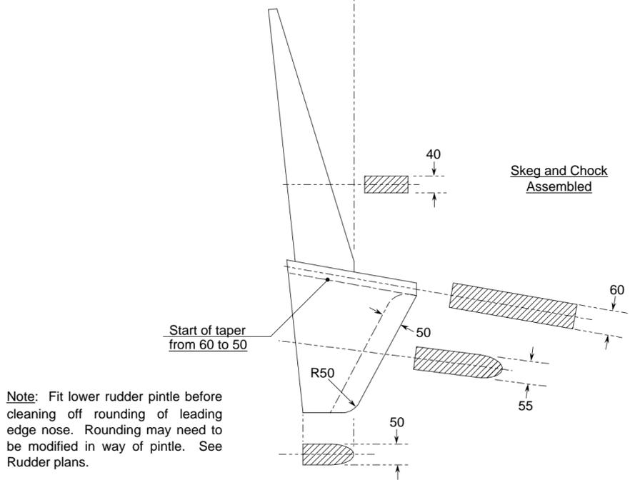
Note: Fit lower rudder pintle before cleaning off rounding of leading edge nose. Rounding may need to be modified in way of pintle. See Rudder plans.
