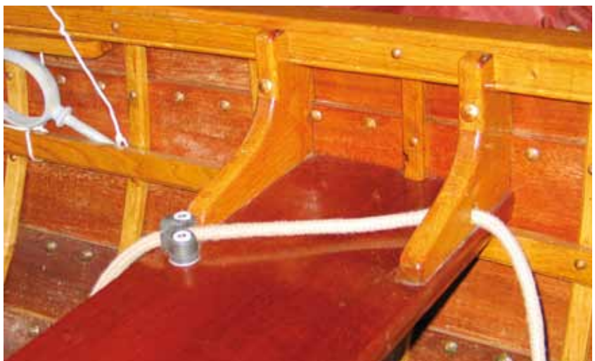
Above: The breasthook is a horizontal knee, made from two arms which were glued together with a hidden tongue. Below: Though the thwart is supported by the risers, the pairs of hanging knees have the important function of bracing the hull athwartships.
