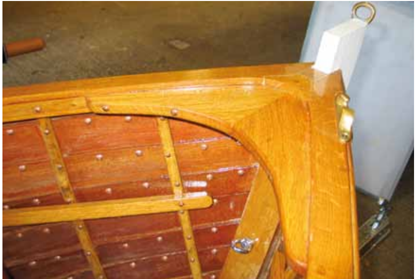
Above: The breasthook is a horizontal knee, made from two arms which were glued together with a hidden tongue. Below: Though the thwart is supported by the risers, the pairs of hanging knees have the important function of bracing the hull athwartships.
