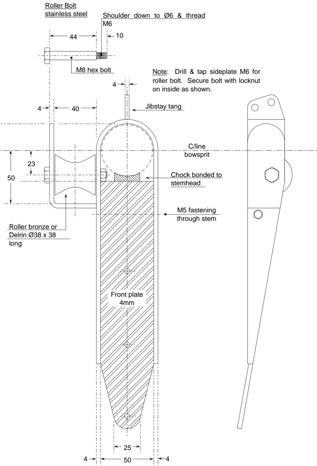
Note: Drill & tap sideplate M6 for roller bolt. Secure bolt with locknut on inside as shown.
