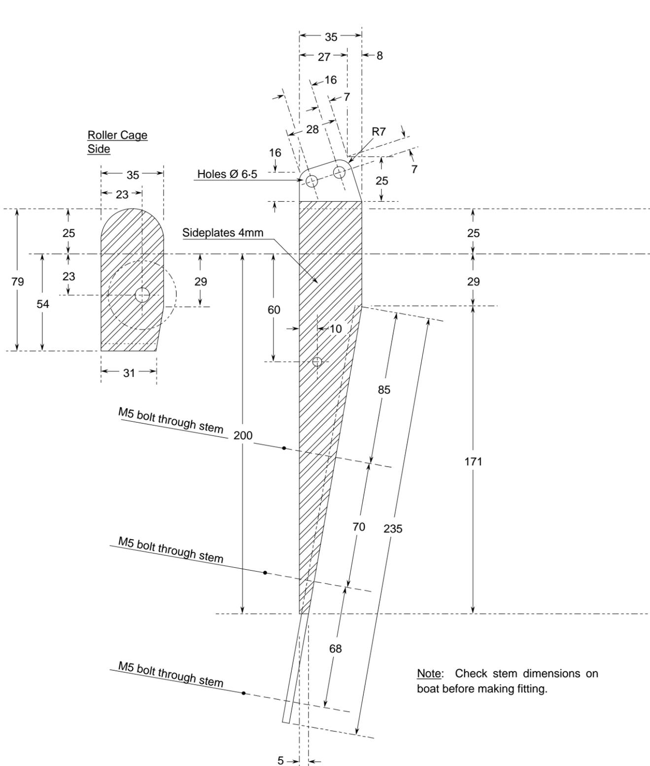
Note: Check stem dimensions on boat before making fitting.
