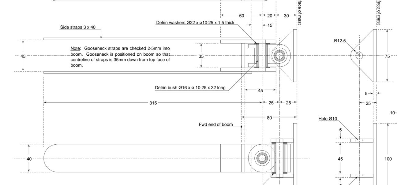
Note: Gooseneck material stainless steel Grade 316 S16, polished finish. Gooseneck made from 5mm material (side straps 3mm and bushes as shown). Delrin for bearing bushes and washers.
