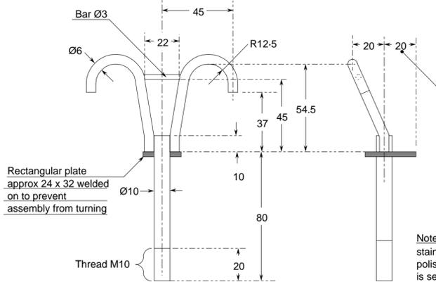
Note: Fitting fabricated from stainless steel Grade 316 S16, polished after fabrication. Fitting is secured by M10 nut & lock-nut.
