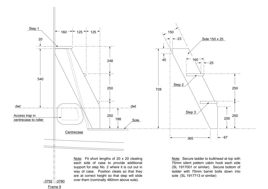
part of ladder which is removable to gain access to engine etc.
