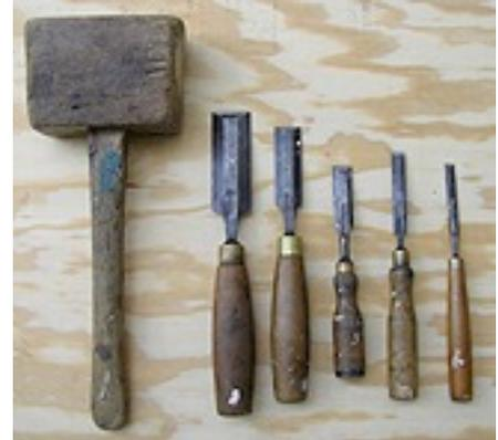
4.5.2. Mortice chisels are a specialized firmer chisel, thicker and narrower, and stronger, for chopping mortices and levering out the choppings.
