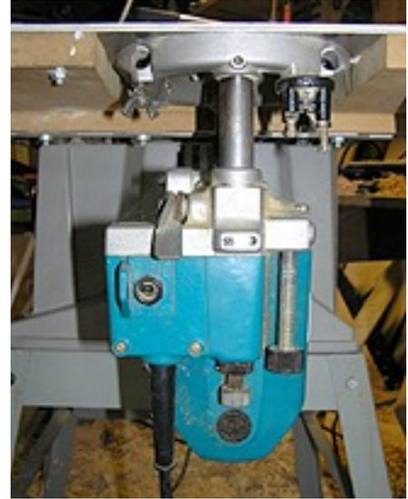
3.9.3. My router here is shown mounted on a home-made table, attached to my table saw. It can use it's own fence or the table saw fences as appropriate.
