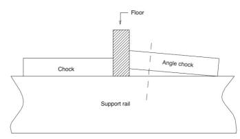
in this case the angled chock is perhaps more secure agains the vibrations of building the boat.
