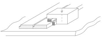
5.7.4. Another example is the angled chock shown opposite, which is pushing the floor up against a chock, so that it is held tight in the correct position. This example is from setting up floors and frames in the building jig on Design 155. You could do much the same job with a flat chock and a pair of folding wedges, but
