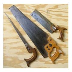
cut each side with the circular saw and then saw the remaining centre portion with the panel saw. And of course you can cut an item in situ, where a power saw would be both difficult and dangerous to use. Many modern panel saws are 'sharp-edge' – that is they have hardened sharp teeth, that cannot be resharpened – but while they are sharp they cut very well.
