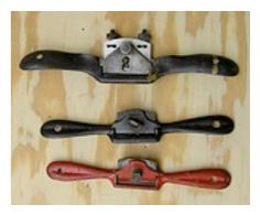
high up on stagings and it broke into three bits! Brazed up like that, it has been serving me well ever since – I actually had to buy a new blade for it recently; the original was completely sharpened away.
