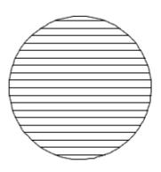
of little use. For boatbuilding purposes, a vertical end grain direction is needed for areas like teak decking as this tends to be the most stable and the grain on the surface doesn't 'shell' out. And reasonably vertical grain is better for items such as the Shelf (Clamp) and for strip-planking. Boards with a more horizontal grain can be used for many general purposes, particularly larger items, such as laminating the hog, laminating the stem, making the keel, sternpost, floors, etc.
