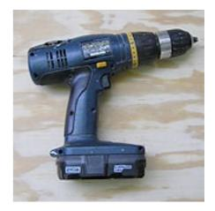
3.3.3. A keyless chuck is almost universal nowadays and, provided it is a good one, very convenient. The chuck on this drill is very good in that it almost
