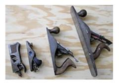
jack plane for straightening the edges of boards. I do however use it quite a lot. I bought it when I was an apprentice boatbuilder in the early 1960's.
