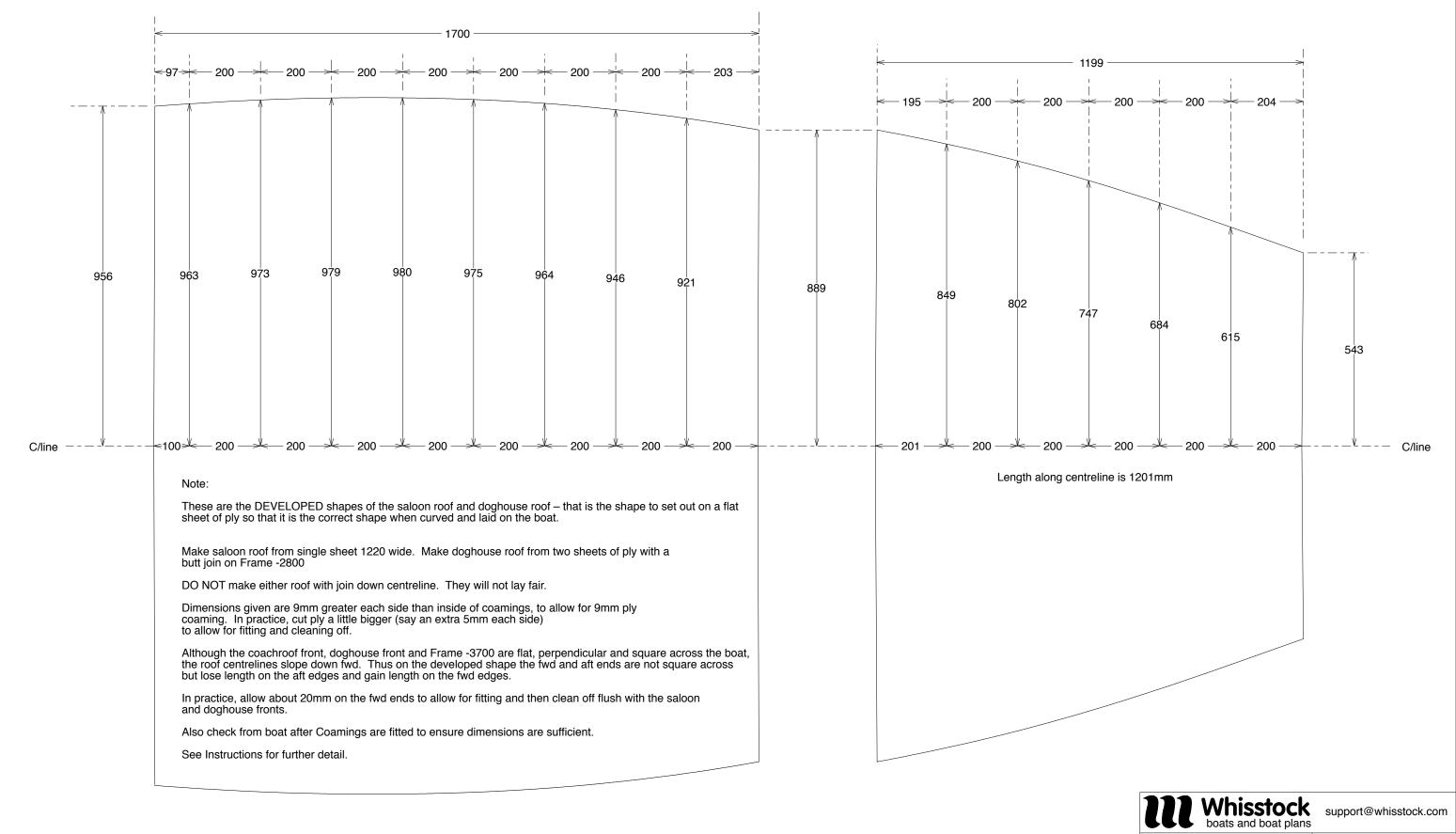
1/10 Scale Design 165 Jul 30 2014 Date Plan No. 165/003/010 Developed shapes of Issue No. 01 Saloon & Doghouse Roofs All dimensions in millimetres unless otherwise noted
