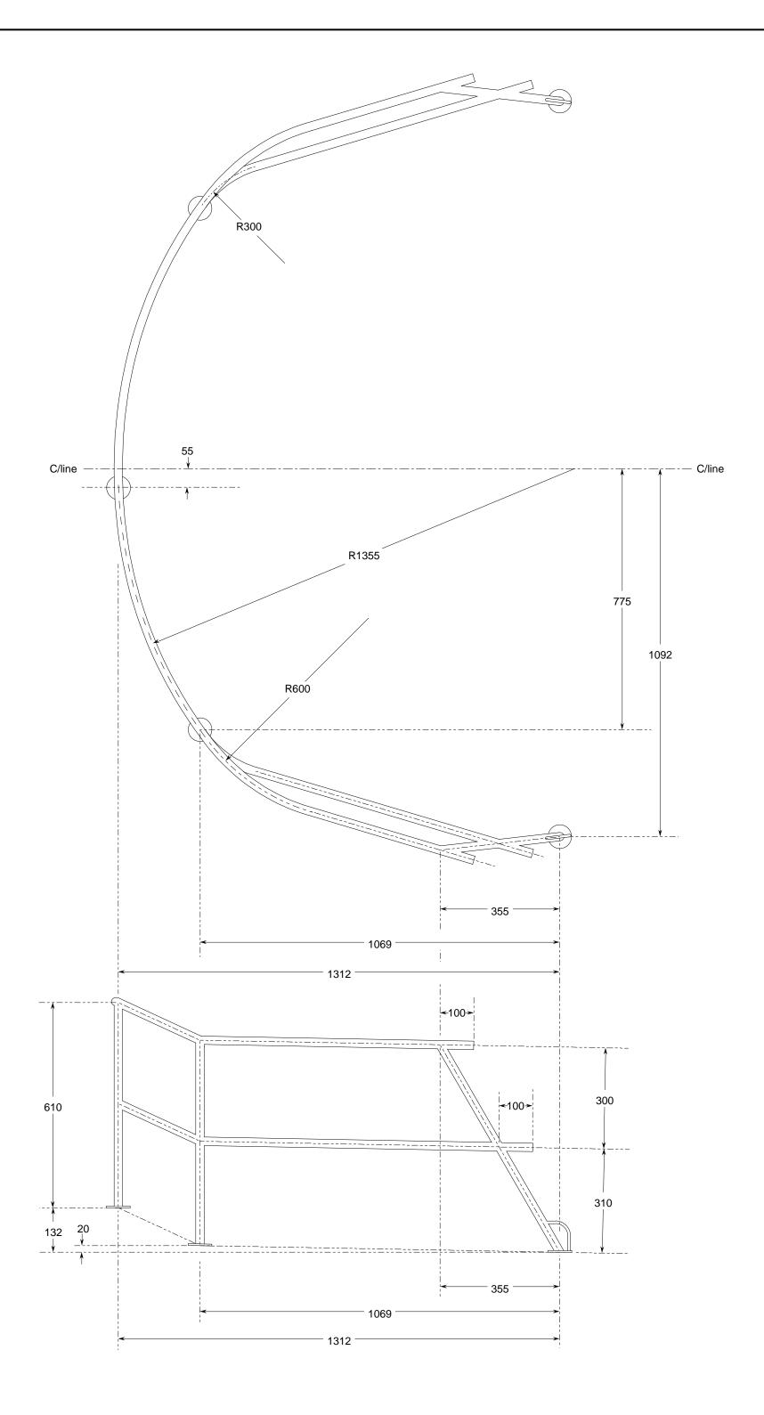
$\underline{\text{Note}}\text{: Stern pulpit is made from } \varnothing 25 \text{ x 1.5mm wall S/steel tube, polished after fabrication.}$
