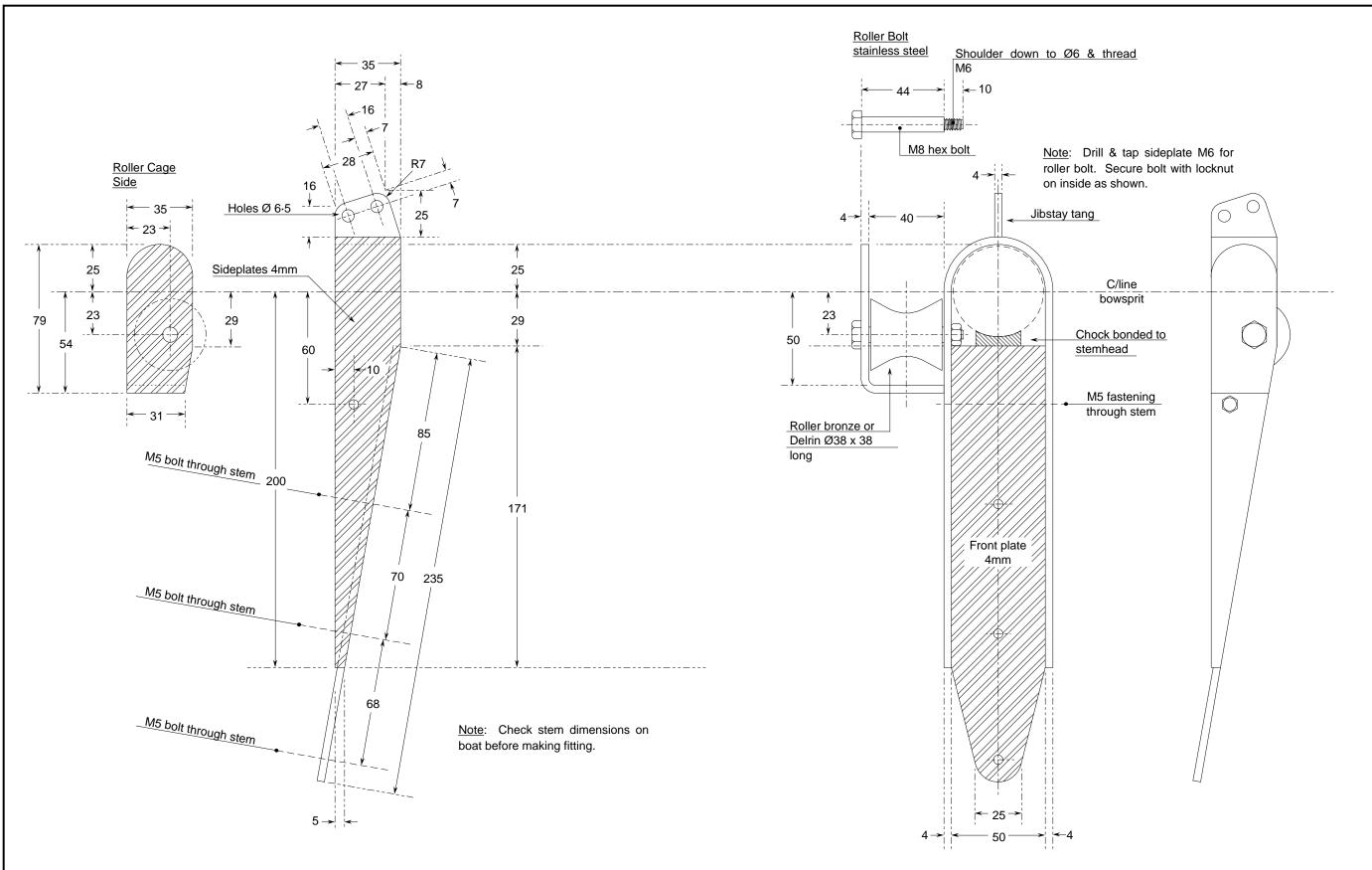
Note: Stemhead fitting is fabricated from phosphor bronze CuSn5 (PB102), TiG welded and polished after fabrication. Or alternatively stainless steel grade 316.
